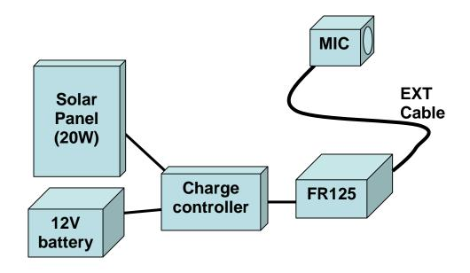
An overnight monitoring station only requires the FR125-EXT, battery, and microphone. Under normal conditions the FR125-EXT will operate up to a week using a 12V 18Ahr deep-cycle battery.
